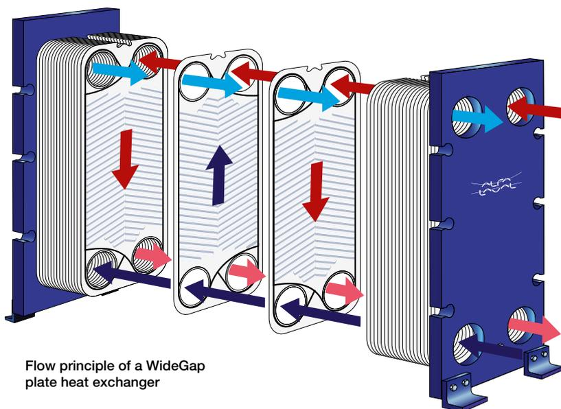
Flow principle of a WideGap plate heat exchanger
